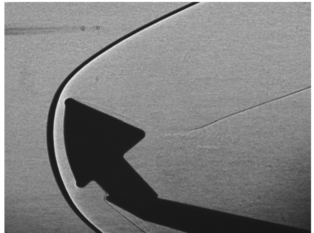
Figure 6-15: Mach 4, Angle of Attack 10 deg, Pt = 12Bar, T0 = 285 K.
