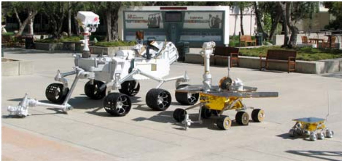
Figure 3-1: Size Comparison of Mars Rovers – from left: Mars Science Laboratory (2011); Mars Exploration Rover (2003); Mars Pathfinder (1996).
