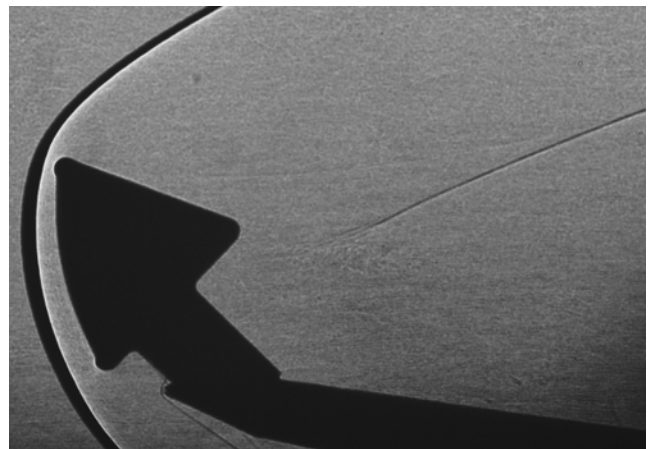
Figure 6-16: Mach 4, Angle of Attack 14 deg, Pt = 12Bar, T0 = 285 K.
